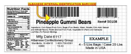
The lot number is defined using the Albanese internal identification barcode. In this example, the lot number is 201006117. The  $\underline{Mfg}$  Date and the last 4 digits of the Albanese internal identification barcode are the Julian manufactured date.
